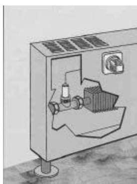
Type 66 Control with Type 61 Straight Valve
