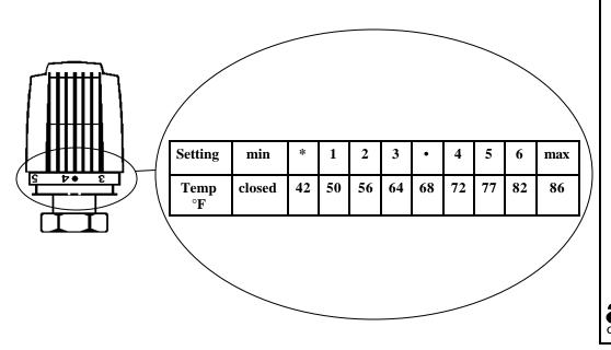
The control's temperature settings may be locked or limited using the following procedure:
