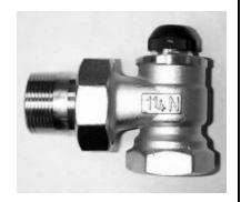
Ammark one pipe steam valves must be installed upright with steam flow in the direction of the arrow on the valve body. Select a control which allows unrestricted flow of ambient room air around the sensor. A mmark control Type 63 remote sensor or Type 66 remote sensor wall/cabinet mount is recommended for optimum efficiency.
